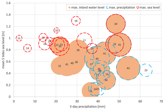
Figure 4. Inland water level anomaly as the difference from the regulated inland water level (cm) for the 15 highest sea level (mean sea level over a five-tide period above NHN (m); red circles) and precipitation (antecedent 3 d precipitation sum (mm); blue circles) events in the 2000–2019 period. Additionally, the 15 highest inland water level anomalies in the same period are shown (orange bubbles). The diameter of the circles is proportional to the size of the difference between the observed and the intended regulated inland water level (number in the circles and bubbles in centimetres).
