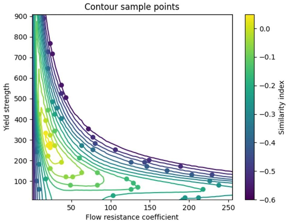
45 **Figure S7: Location of the flow mobility samples that produce the maps used in the expert assessment of half degraded performance (Fig. S6). Contours and colors map the similarity index of the response surface displayed in Fig. S5.**
