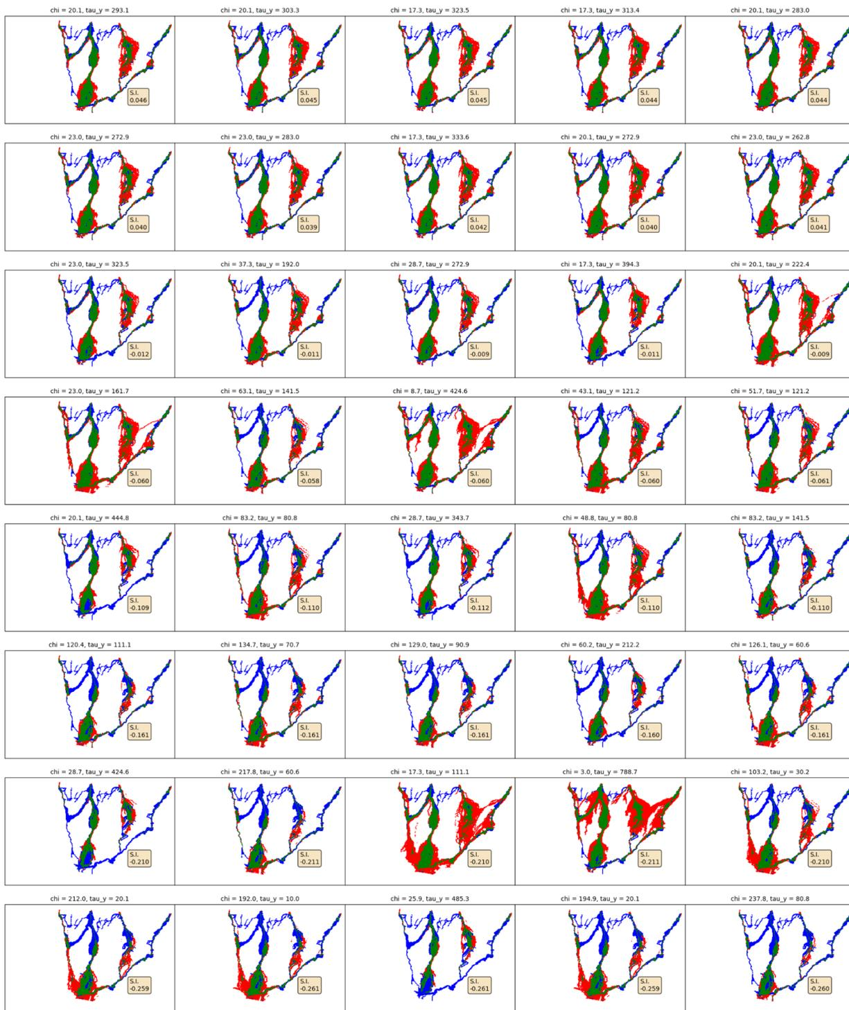
**Figure S6: Inundation maps used by experts (see S1) to determine the similarity index contour level of half degraded performance. In each plot, green = True Positives, blue = False Negatives, and red = False Positives.**
