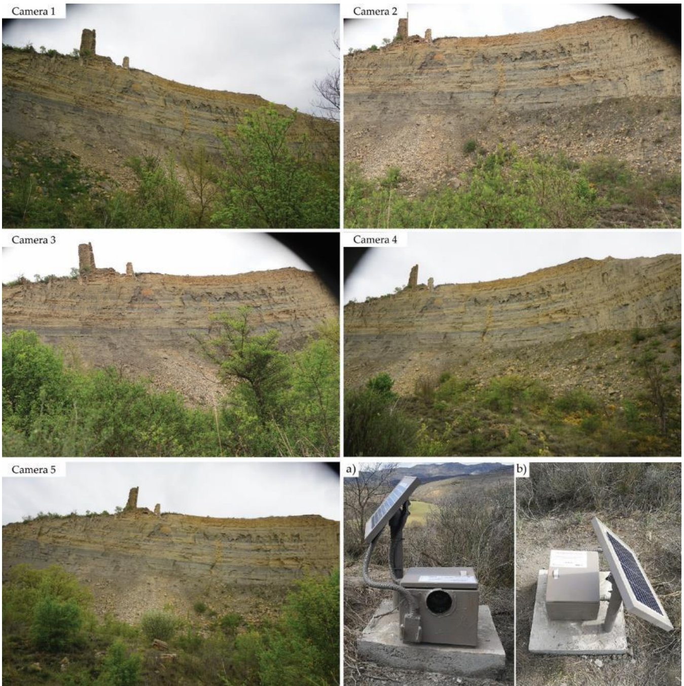
Figure S6. Images obtained with each high resolution photographic module installed in Puigcercós on 22 April 2019 at 17:47h. Three cameras use the Sony Alpha 7R III with a resolution of 42.4 MPx and are equipped with a 35mm f/2.8 lens. The other two modules use a Canon 77D DSLR camera with an APS-C sensor and a resolution of 24.2 MPx. The Canon cameras are equipped with a 24 mm f/2.8 pancake lens. a,b) images of the modules installed in the field.
