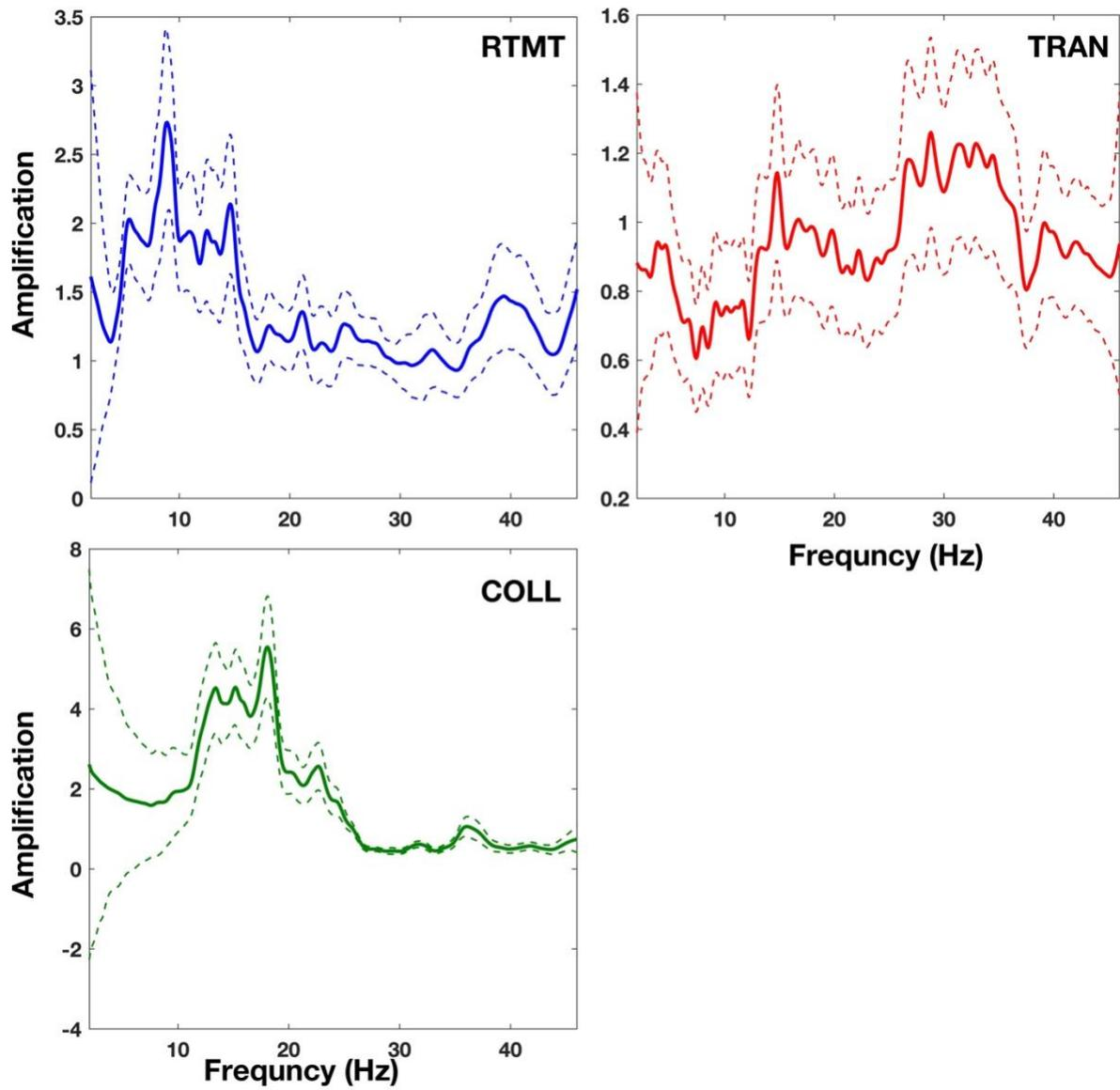
Figure S4. H/V ratios for each of the three stations along the Whangaehu channel. Solid lines represent the average H/V ratio from all computed time windows. Dashed lines represent the standard deviation of all the H/V time windows.
