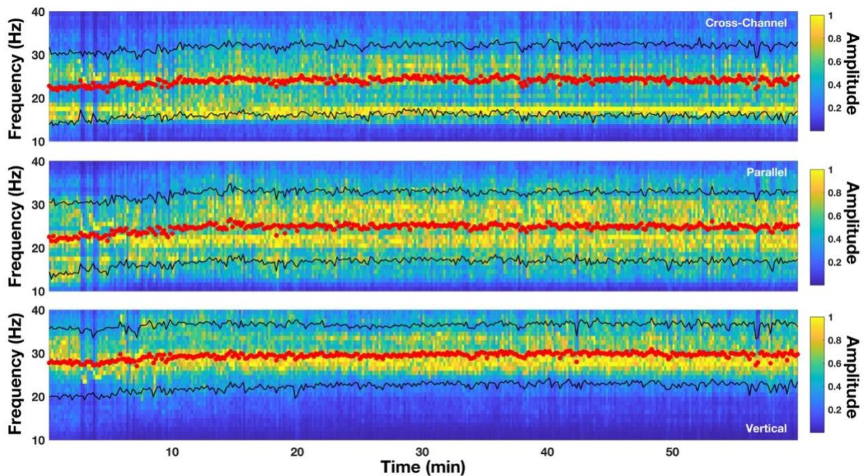
Figure S3 Normalized spectrograms for COLL. Red dots represent the spectral centroidal frequency and black lines show the range of the spectral spread.
