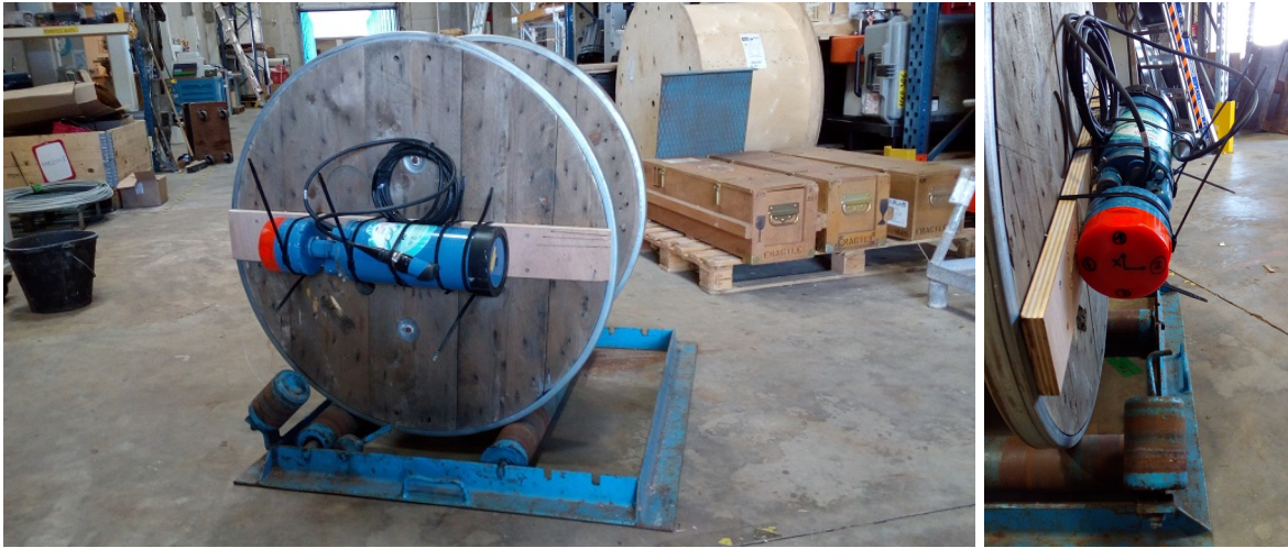
Figure S1. Photos of system used showing the position of the device for an applied X-tilt of -90^\circ (X-axis vertical up)
