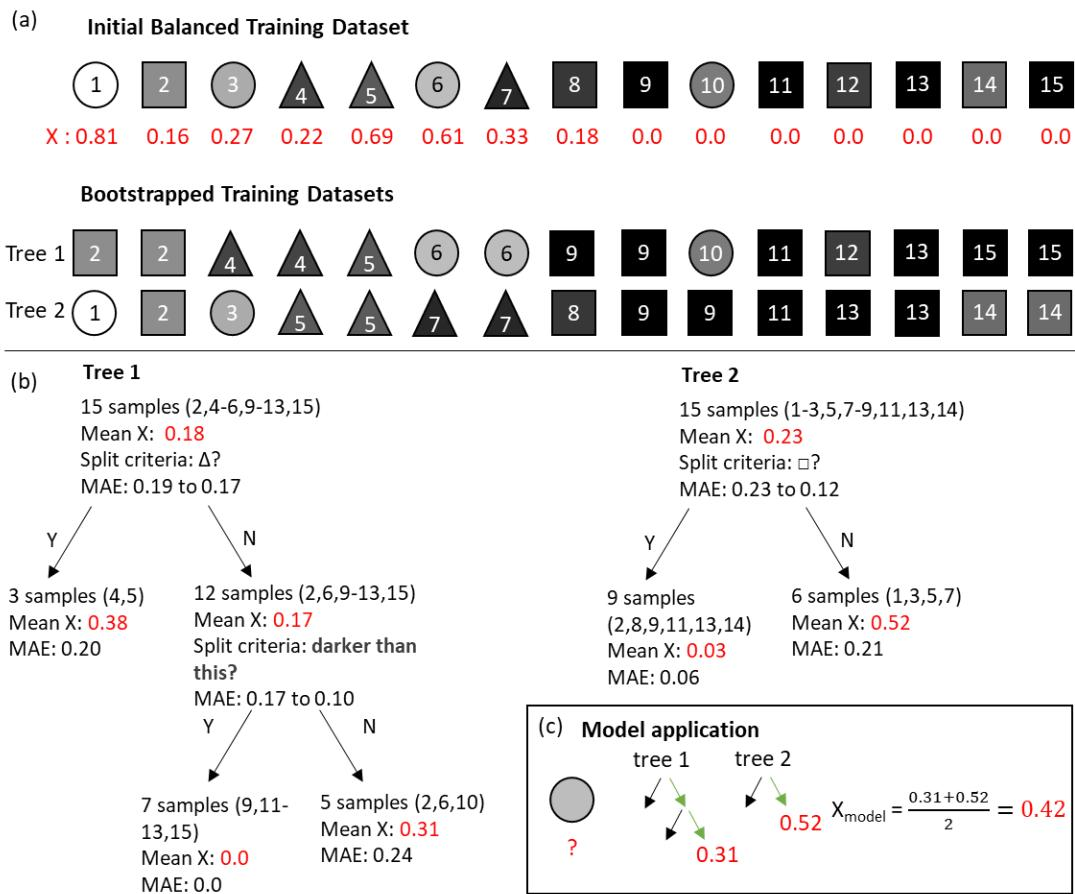
A simple example of the Random Forest Regression technique (developed by Breiman, 2001). Here two trees are used to estimate the value of X a sample should be assigned based on two input features: the colour and shape of each sample. Tree 1 has a “depth” of 3, while Tree 2 has a “depth” of 2.
