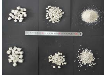
(c) Sieved granules of different particle sizes
