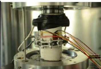
(b) Standard specimen under a uniaxial compression test
