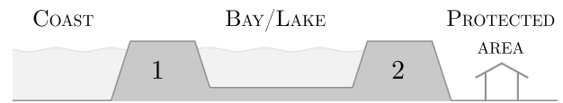
Figure 20. A coastal system with two lines of defence. This figure is an adaption from an illustration found in Dupuits et al. (2017).
