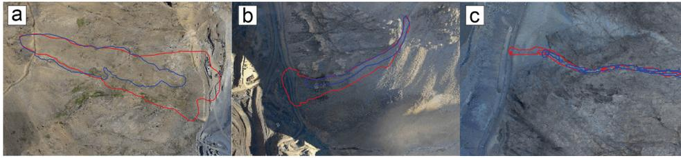
**Figure 15.** Comparison between avalanche runout distance using cold ( $T_0 = -10\text{ }^{\circ}\text{C}$ , blue line) and warm snow ( $T_0 = 0\text{ }^{\circ}\text{C}$ , red line) for the (a) LGW-2, (b) BN-1 and (c) CCHN-3 case studies. Warm snow leads to more frictional melting and longer avalanche runout.
