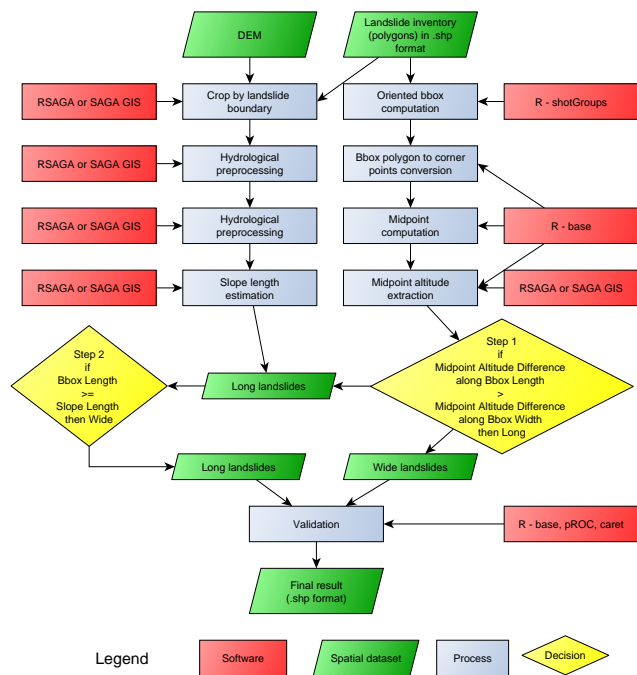
Figure 4. Workflow of the proposed algorithm implemented as an R script.
