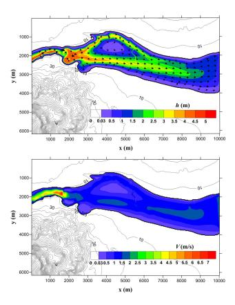
**Figure 6.** Snapshots from the application of FLOW-R2D in the estuary of Spercheios River with water depth and flow velocity, respectively.
