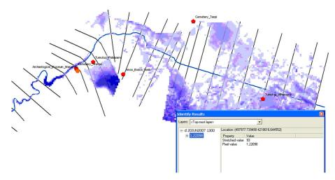
Figure 3. The flood hazard map of Rapentoza watershed for the scenario of T = 100 years (blue colour indicates the inundation area).
