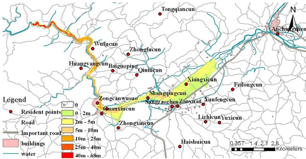
Fig. 9. Flood inundation potential analysis (5.19 full break).
