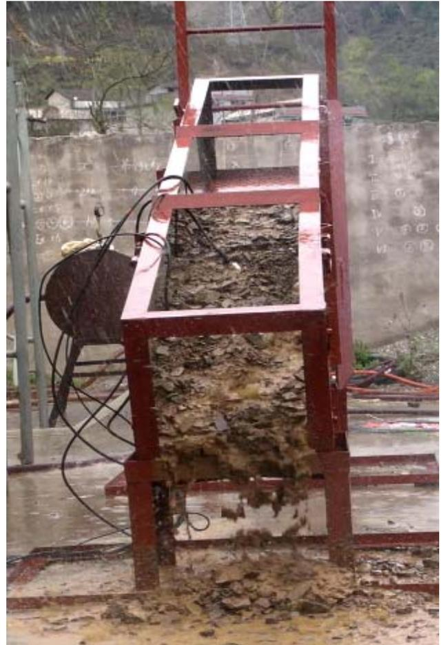
**Fig. 6.** Soil slides down sharply and landslide occurs.
