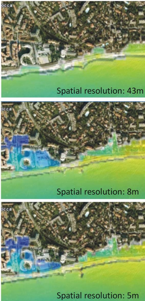
**Fig. 3.** Detail of the different inundations computed with the same initial conditions and input parameters, changing only the spatial resolution of the DTM (Cannes test site, south of France). Simulations have been performed with COMMIT (Cornell University), in the frame of the French ANR “MAREMOTI” project.
