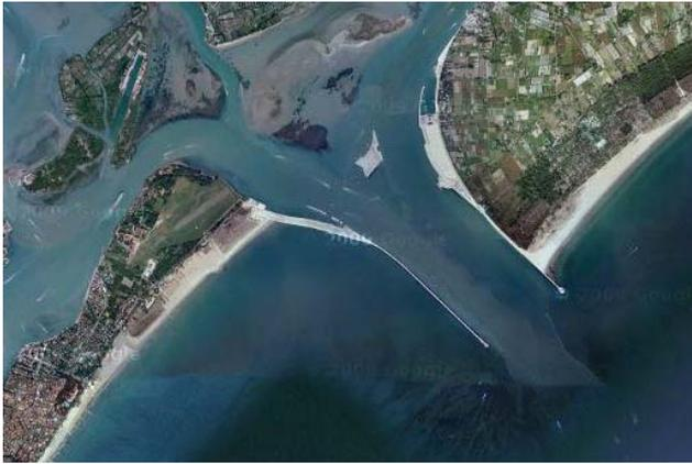
**Fig. 13.** The Lido inlet to the Venice lagoon. The length of the jetties is about 2 km.
