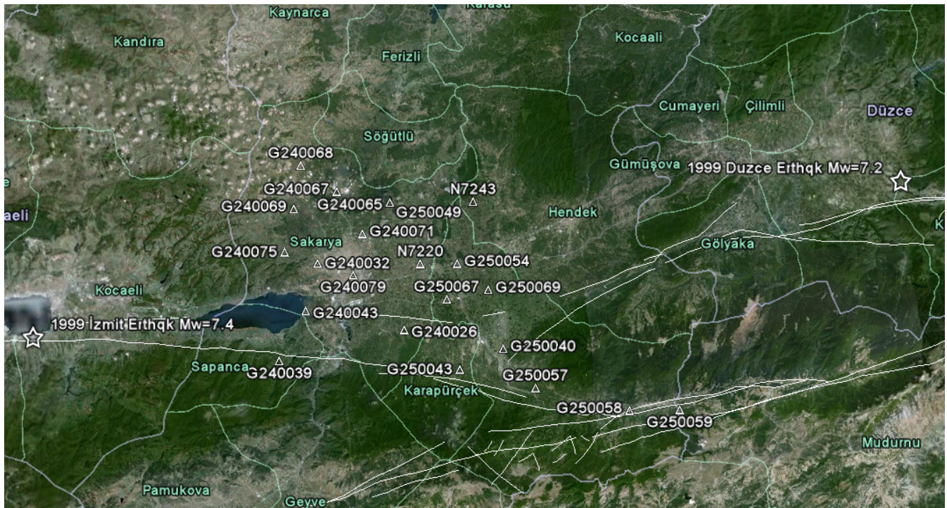
Fig. 4. Sakarya geodetic control network. Triangles display the network control stations. Stars show the location of the earthquakes. Solid white lines represent the fault lines (satellite image from Google Earth).
