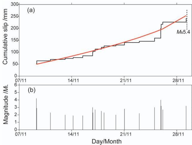
**Fig. 6.** (a) Power-law fit of the pre-shock cumulative slip curve, for the “repeaters” within the Xiuyan 52-plet, occurred before the Xiuyan earthquake. The power-law curve is represented by the red line, showing the accelerating-like behavior. This figure is a further zooming-in of Fig. 5a and b. (b) Magnitude-time plot of the “repeating earthquake sequence” in (a). It is somehow similar to foreshock activities, but the spatial range is limited to the range of the “multiplet”.
