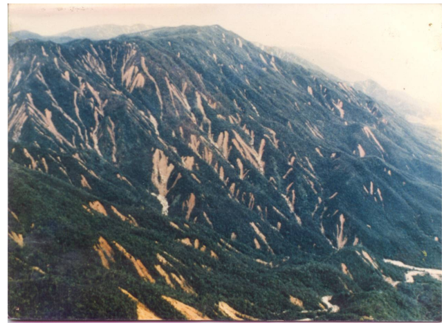
Fig. 2. Landslides triggered in Serra do Mar during a heavy rainfall (379.4 mm/48 h) in 1985. The occurrence of mass movements is common in this region, mainly shallow landslide types (Archive: Technology Research Institute of the São Paulo State/IPT).
